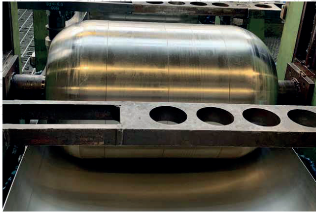
Pipes from Coil (Continuous Process) (3 Coil Lines – OD 3" to 20" – WT 2 to 13mm)
